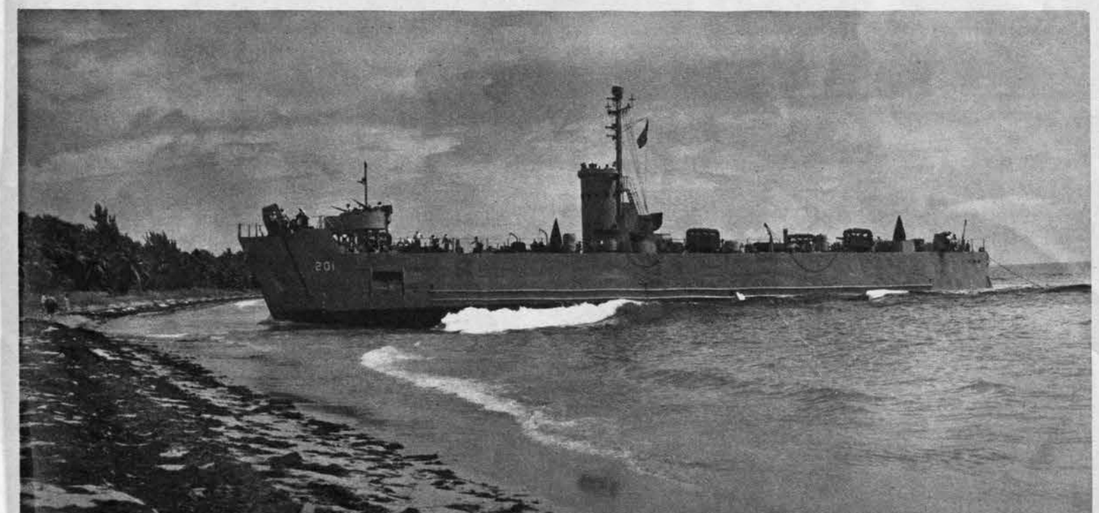
Landing ship, medium (LSM) is a large vessel roughly resembling the familiar LCI. Unlike the LCI, she does not have the troop gangways overhanging the hull. Instead she has an expansive well extend-
